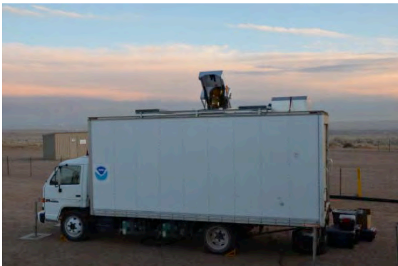
5-3. Truck-mounted TOPAZ ozone lidar with roof-top, two-axis scanner.
