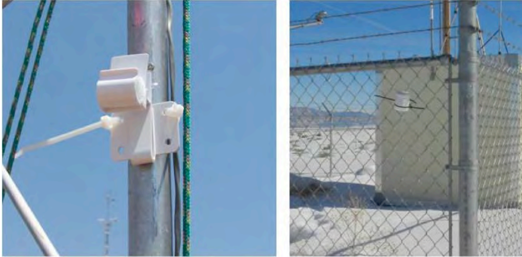
5-4. Deployed Ogawa passive sampler without and with rain/wind cap.
